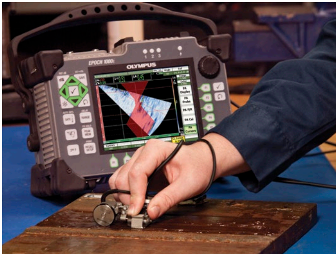
Phased Array S-scan with Weld Overlay
