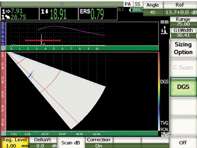
Phased Array DGS/AVG Mode
